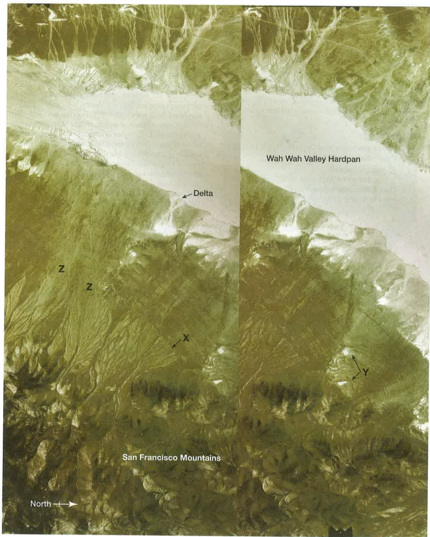
FIGURE 14.8 Stereogram of the Wah Wah Valley, Utah, area: 1:58,000 scale. The stereogram is constructed with two 1991, National high-altitude photograph (NHAP) aerial photographs (Courtesy of U.S. Geological Survey). View this stereogram using a pocket stereoscope (FIGURE 9.9, page 241) or by crossing your eyes. Hold the stereogram at a comfortable distance (one foot or so) from your eyes with your nose facing the line between the images. Cross your eyes until you see four photographs (two stereograms), then relax your eyes to let the two center photographs merge into one stereo image.
